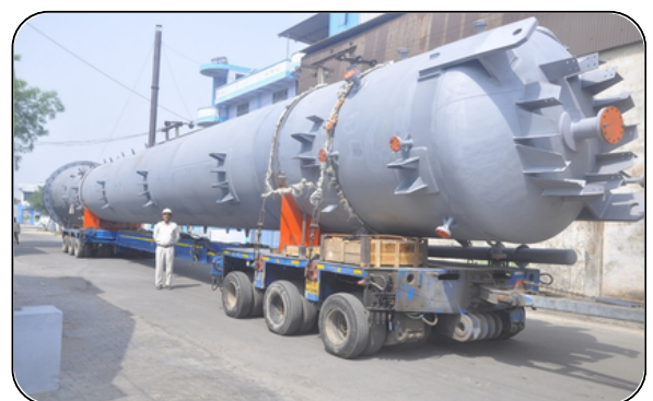
Caustic Wash Column
